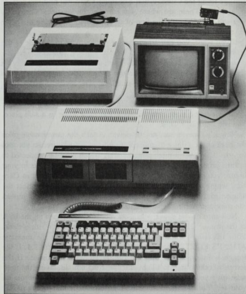
Figure 1.3: The full Adam system consists of the computer console, the printer, the television, and the keyboard.
